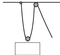
*A pulley uses wire/rope moving on a grooved wheel. One or more wheels can be fixed or moveable.*
