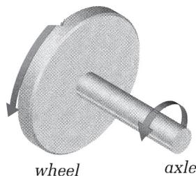
***It is two wheels of different diameters that turn together. A longer movement on the wheel produces a shorter but more powerful motion at the axle. In the other direction (force applied to the axle) it is used to increase speed.***
